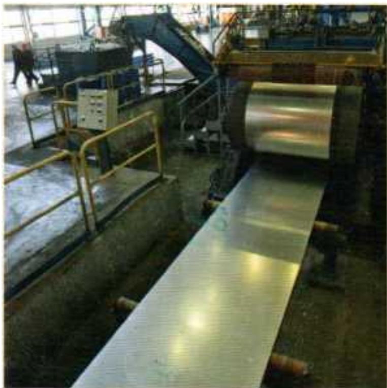
Figure 11.10 Sheets of metal are coated with zinc in this iron and steel works in Russia to stop it rusting.
