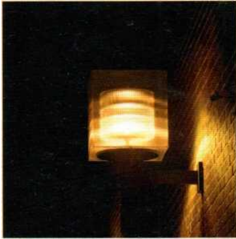
Figure 11.3 Electricity heats the sodium until it changes into a gas called a vapour and gives out an orange-yellow glow.
