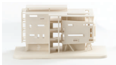
Figure 2.7 A prototype produced on a 3D inkjet printer
