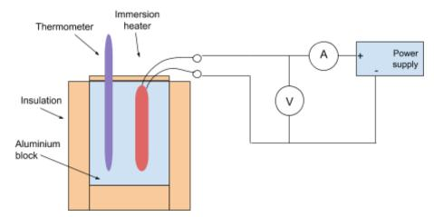
Below is a diagram for an experiment finding the specific heat capacity of aluminium:
