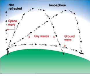
Figure 7-1. Ground, space, and sky wave propagation.
