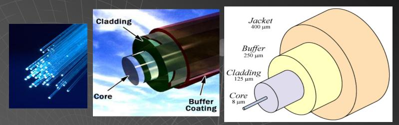
A single optical fibre, will have the following parts:
