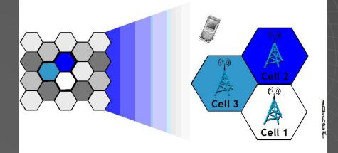
Although each cell is approximately circular (depending on the flatness of the land), the cells are shown as a 'honeycomb' so that the cells fit together.
