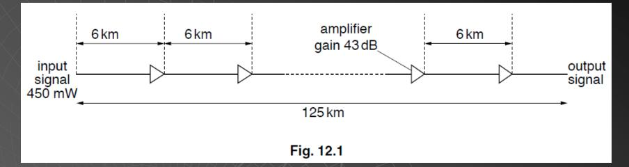
A signal is to be transmitted along a cable system of total length 125 km. The cable has an attenuation of 7 dB km–1. Amplifiers, each having a gain of 43 dB, are placed at 6 km intervals along the cable, as illustrated in Fig. 12.1.
