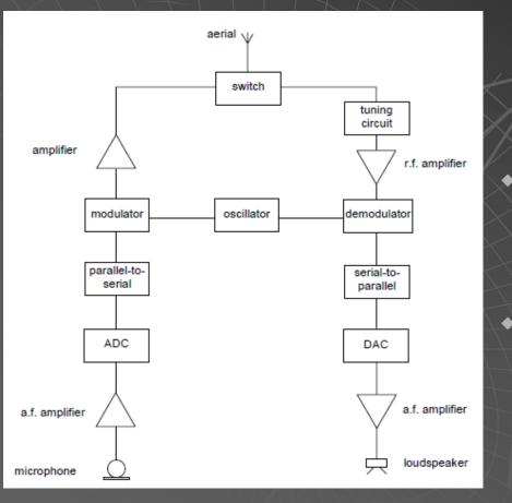
On receipt of a signal at the aerial, the signal is switched to a tuning circuit that selects only the carrier-wave frequency allocated to it by the computer located at the cellular exchange.
