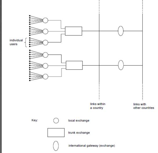
In essence, the Public Switched Telephone Network (PSTN) uses the same principles of exchanges but has developed with modern technology and the number of users.
