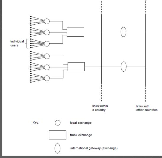
The user is connected to the PSTN via the local exchange.
