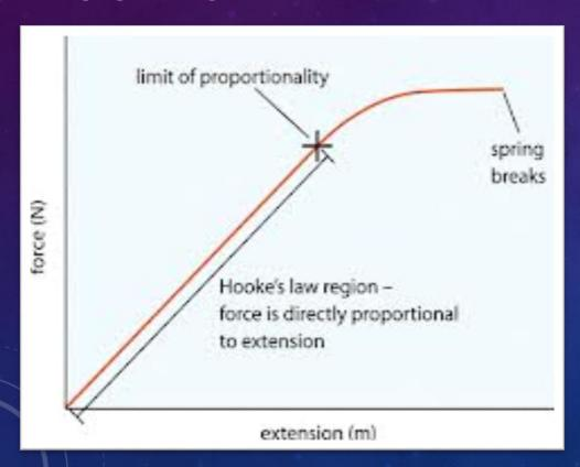
The extension of a spring is proportional to the load applied to it, provided the limit of proportionality is not exceeded.
