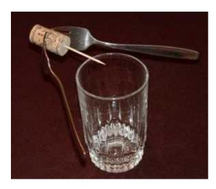
For an object to be in stable equilibrium, a vertical line down through its centre of gravity must run within the boundaries of its base; if tilted until this line falls outside the base, the object becomes unstable and topples over
