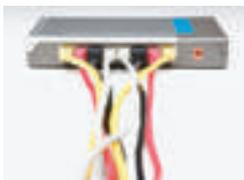
**Network hubs** are hardware devices that can have a number of devices/computers connected to them. Its main task is to take any data received via one of the ports and then send out this data from all of the ports. Each computer/device will receive the data, whether it is relevant or not.
