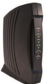
**Dial-up modems** operate at transmission speeds of about 60 kilobits per second, which is quite slow by today's standards. (These are discussed in more detail in Section 4.4.) However, modern broadband or **asymmetric digital subscriber line (ADSL)** modems operate at 11,000 kilobits per second (or higher). The term 'asymmetric' means that the modem is faster at **downloading** (getting) data than it is **uploading** (sending) data.
