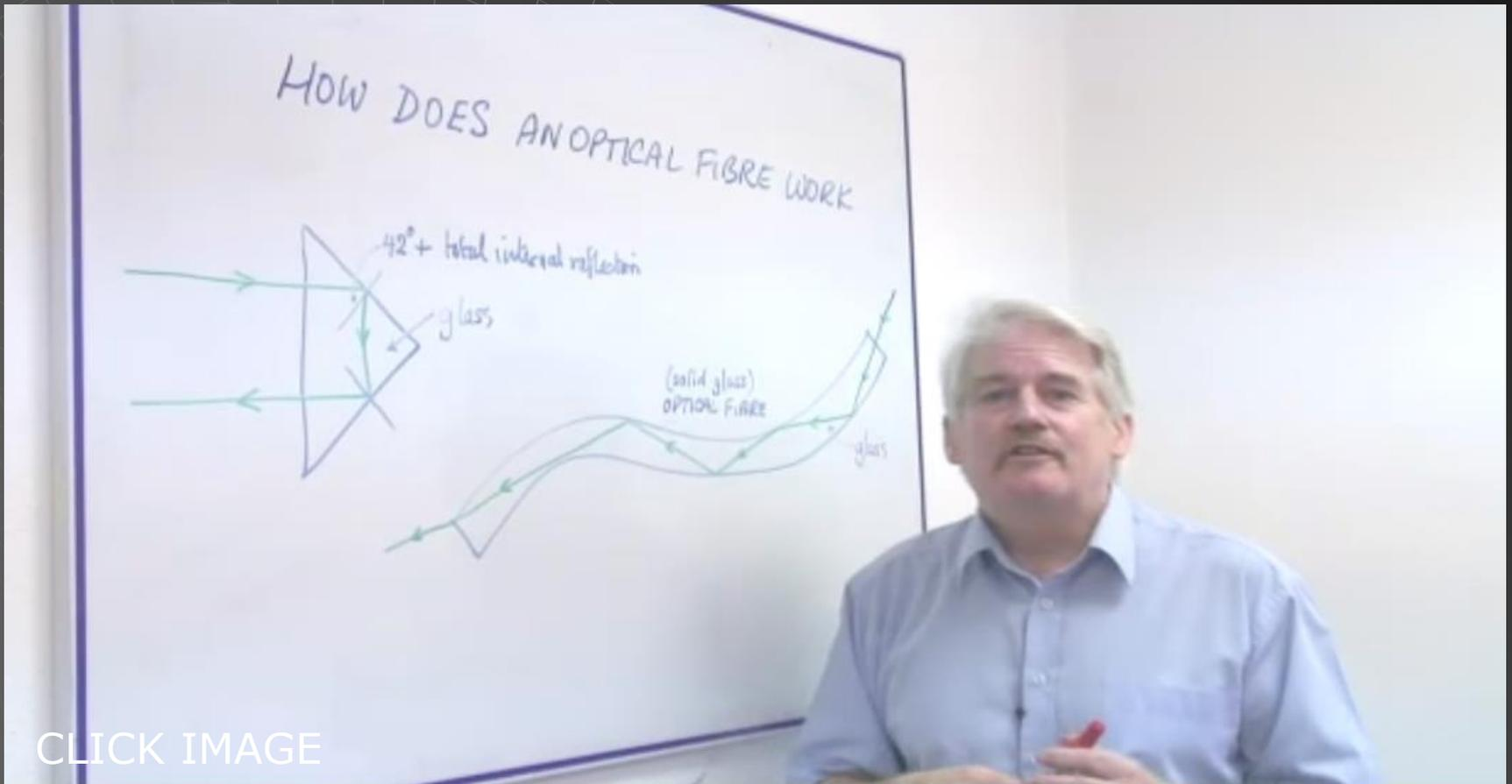
Optic fibres transmit optical pulses using the principle of total internal reflection.
