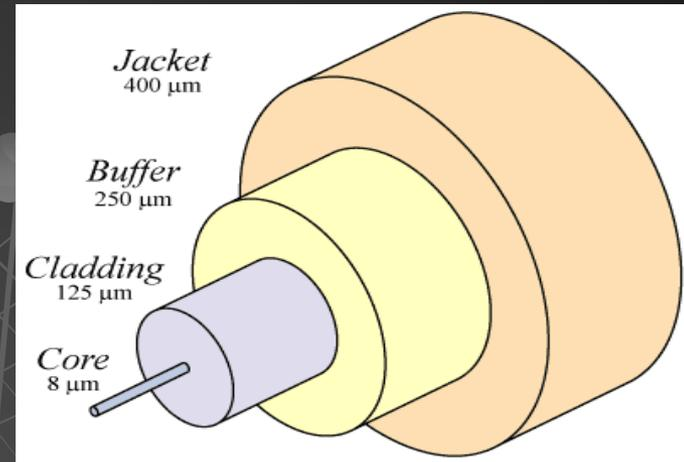
**A single optical fibre, will have the following parts:**
