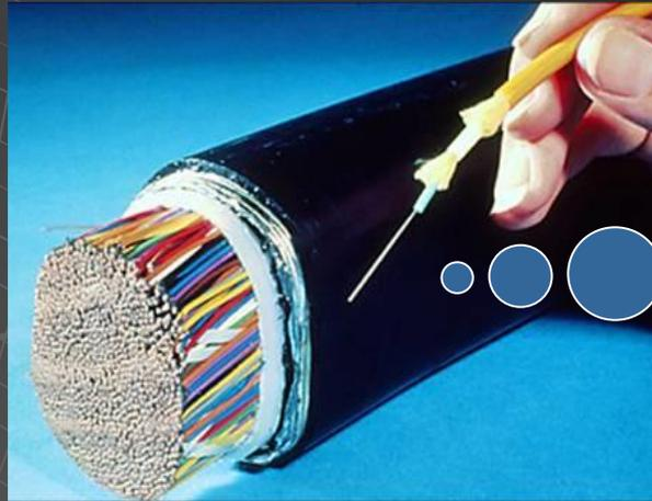
One single optic fibre can transmit as much data as a bundle of coaxial wires
