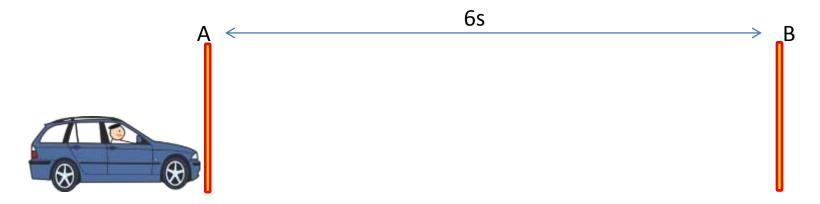
Car passes point A with a velocity of 10m/s. It has a steady (constant) acceleration of  $4m/s^2$ . What is the velocity when it passes point B?
