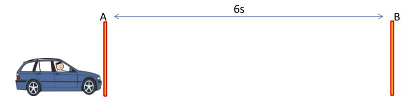
Car passes point A with a velocity of 10m/s. It has a steady (constant) acceleration of 4m/s<sup>2</sup>. What is the velocity when it passes point B?
